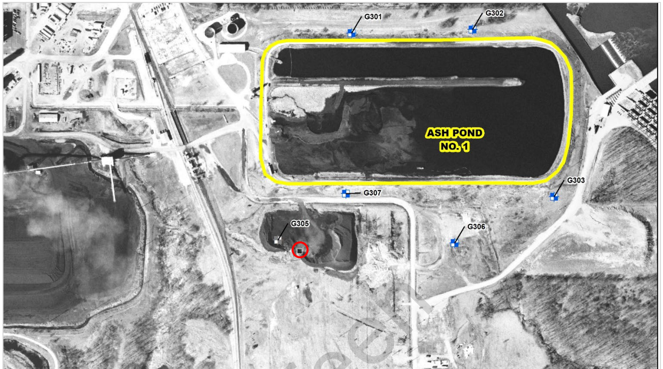
Figure A. Coal Storage Near AP1. An aerial photograph from April 2005 shows potential coal storage near G307 and G306, and a mine shaft (black box, circled in red) near G305. Groundwater generally flows from the southwest to the northeast across AP1 (ISGS, 2018b).
